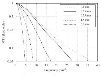
Fig. 3. MTF as a function of crystal size.
