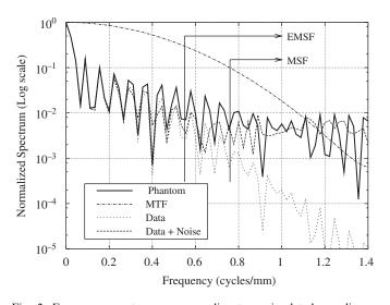
Fig. 2. Frequency spectrum corresponding to a simulated one-dimensional case. The frequencies of the noise-free acquisition correspond to the product of the frequencies of the phantom and the MTF of the tomograph. It can be noticed that in the noisy data those frequencies higher than the EMSF are dominated by noise.
