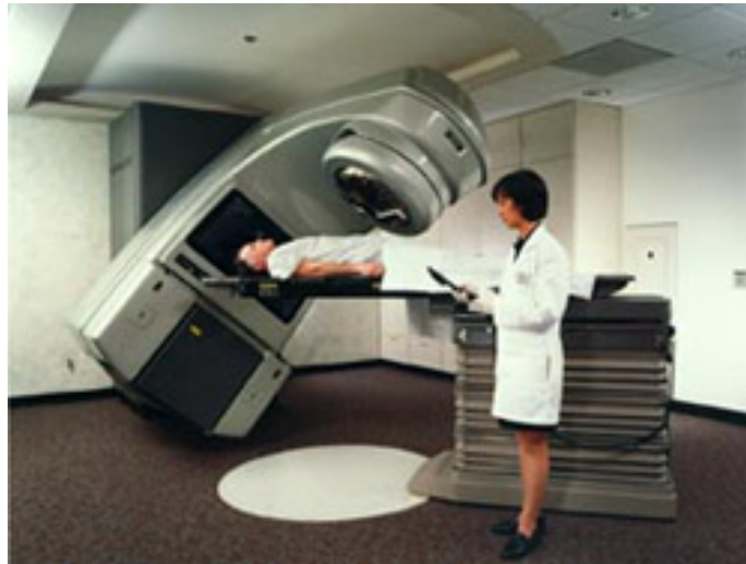
Figure 1 A modern 3 GHz linear accelerator used for photon and electron treatments rotates around the patient, so that the beam can be directed to the target from any direction.
