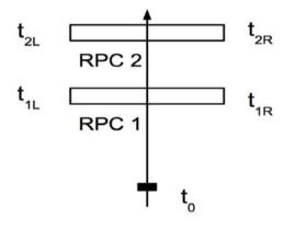
$$\sigma_{ToF} = \frac{1}{2} \sqrt{\sigma_{t_{1L}}^2 + \sigma_{t_{1R}}^2 + \sigma_{t_{2L}}^2 + \sigma_{t_{2R}}^2}$$
