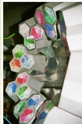
MINIBALL (8 cluster of 3 segmented Ge crystals).
