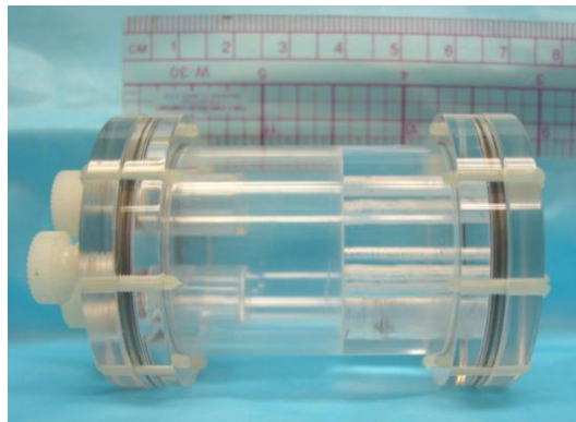
Figure A.2. NEMA NU 4 Image quality phantom.
