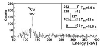
FIG. 2. Particle  $-\gamma$ -ray coincidence spectrum obtained with 6<sup>-</sup> beam of <sup>70</sup>Cu. The spectrum is Doppler corrected for mass A = 70. Upper right corner: partial level scheme of <sup>70</sup>Cu taken from Ref. [12].
