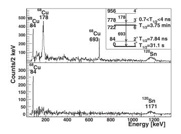
FIG. 1. Top: particle– $\gamma$ -ray coincidence spectrum acquired with the 6<sup>-</sup> beam of <sup>68</sup>Cu. The partial level scheme and deexcitation  $\gamma$  rays shown in the upper right corner are based on Refs. [15,21] and this work. Energies are given in keV. Levels drawn with thick lines represent the  $\beta$ -decaying states. Bottom: particle– $\gamma$ -ray coincidence spectrum acquired with the 1<sup>+</sup> beam. No Doppler correction was applied to these spectra.
