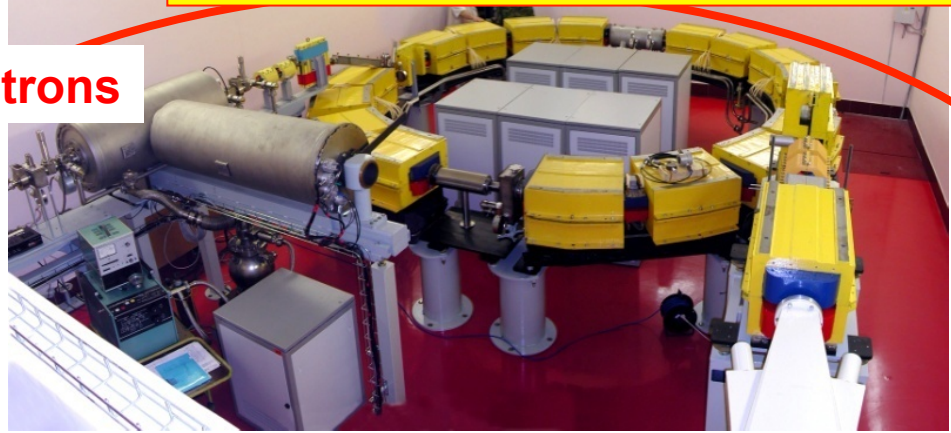
Compact synchrotron (Protom) + Hitachi, Mitsubishi, Toshiba,...
